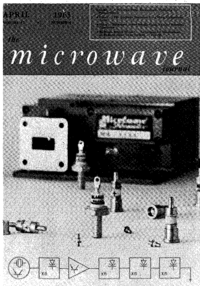
Fig. 4. Cover of the Microwave Journal of April 1963. An X-band varactor-generator source is shown in the background. Various varactors are shown in the foreground. The block diagram across the lower part of the picture shows how these devices are organized.
